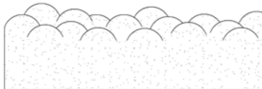
Fig. 5.2: Simplified surface roughness for the Greenwood & Williamson model.
