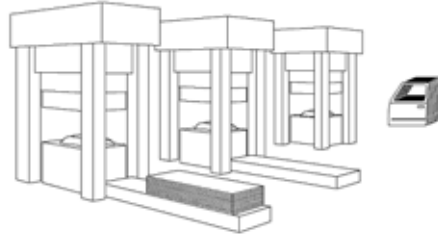
Fig. 1.4: Schematic illustration of a deep drawing press line.
