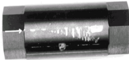
Fig. 2.10: Adhesive wear: transferred zinc lumps on a tool surface.
