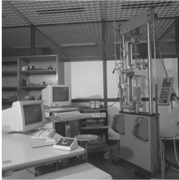
Fig. C.4: Deep drawing simulator - overview of the set-up.
